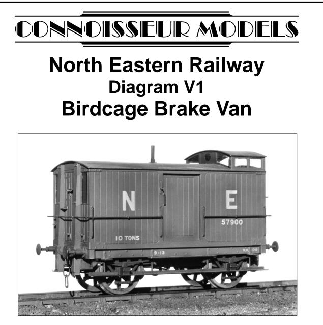
**Prototype.** The diagram V1 brake vans were built by the NER about 1890 -1898. They were a development of similar outside framed vans of much earlier origins and can be thought of as the first standard NER brake van design. They worked in traffic into LNER days and some vans were very long lived with four making it into preservation. A fully restored example is at Beamish Museum.
